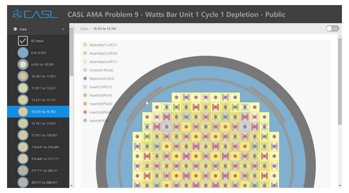
The Core 2D views show the complete reactor at a particular elevation, including the vessel, baffle and neutron pads, if they are included in the input file. The assemblies are each assigned unique colors, shown in the legend on the left side. The controls, detectors and inserts are overlaid on top of the assemblies using circles and bars, to show how they combine in a single location at each elevation.
