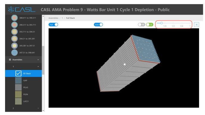
The scale slider. Reduces the vertical scale of the model. Since assemblies or reactors are often tall compared to their width, scaling their height can make viewing and interacting easier.
