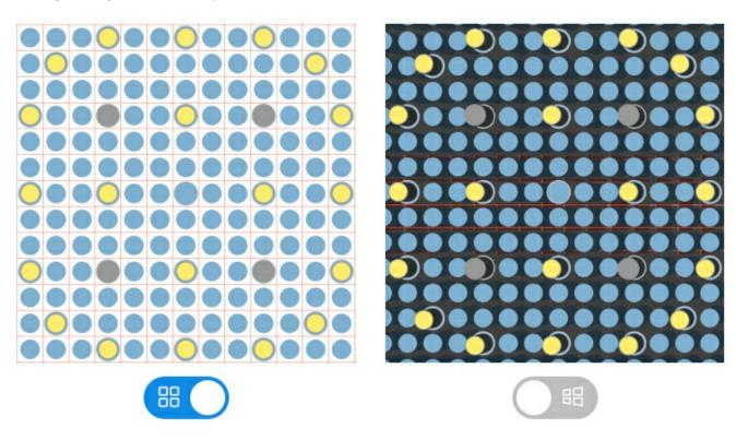
Perspective/Orthographic toggle. Use a realistic perspective view for the camera, or use an orthographic view, which preserves lengths at different distances from the camera. The Orthographic representation would be similar to the 2D view but with a more realistic look.
