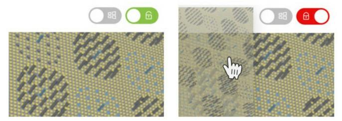
View lock toggle. When this toggle is activated, it takes the current view and makes it into a static image, which can be right-clicked to get the 'Save image as...' option to export the image. It can also be dragged directly to the desktop to save the image as download.png. The view cannot be changed until this toggle is turned off. Note that the image has a transparent background, making it easy to embed in presentations as desired.
